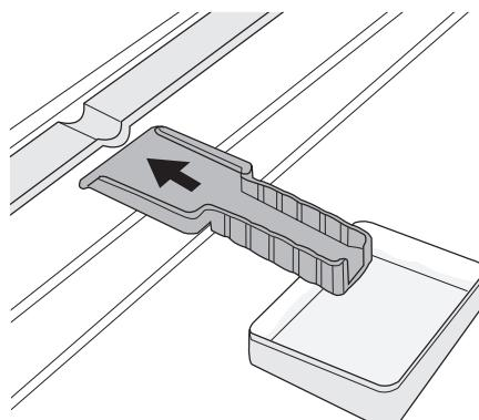
4. When defrosting is completed, dry the interior thoroughly and keep the scraper for future use.
